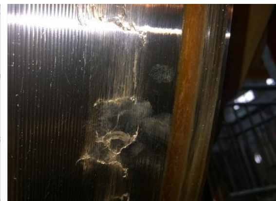
Crack with 80mm length and 25mm width, 11mm below the wheel rim tread
